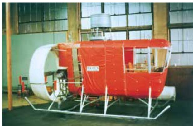
The fan for pressurizing the hull is located beneath the burners to provide an adequate supply of air for propane combustion. The fan is driven by a seven-hp, four-cycle engine. Since pressurization is important for controllability of the airship, a redundant drive for the fan is employed. A clutch engageable power take-off drive from the propulsion engine is used for this purpose.
